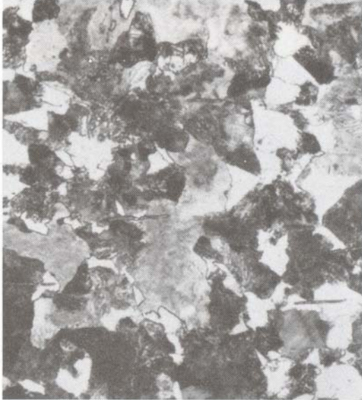
Fig. 163 25-mm (1-in.) diam 4140 steel bar, austenitized 1 h at 845 °C (1550 °F), cooled to 650 °C (1200 °F) and held 1 h for isothermal transformation, then cooled to room temperature. White areas are ferrite; gray and black areas, pearlite with fine and coarse lamellar spacing. Nital. 500×
