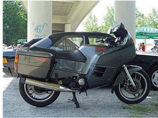
Norton Commander. Engine 588 cc water-cooled twin-rotor Wankel engine Power 85 bhp (63 kW)
