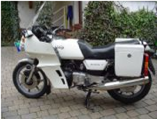
Norton Commander. Engine 588 cc water-cooled twin-rotor Wankel engine Power 85 bhp (63 kW)
