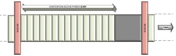
A frame transition can include more than one allocation slots and must not necessarily starts or ends on an allocation slot boundary
