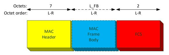
• The MAC header and the Frame Check Sequence (FCS) have fixed-length, and the MAC frame body has variable length
