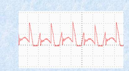
The input to the ADC from the voltage sensor.
